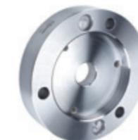
The mounting flange for cylinders with short taper is available in taper sizes 5, 6, 8, and 11. The threaded connection is available in sizes ISO 702-1 (DIN55026, threaded connection), 701-2 (DIN55029, camlock) and 702-3 (studs with nuts). The flanges also fit on the CoAE with center mount.
