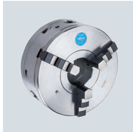
Even more precision is available with our plane spiral chuck in Hi-Tru design. With an adjustment accuracy of up to 0.005 mm, each jaw can be adjusted separately using a separate spindle.
