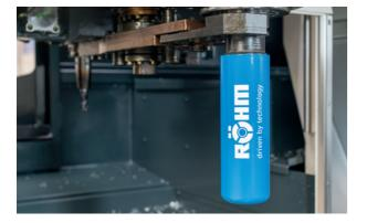
After the lubrication process, Lubritool® is sent back to the tool magazine and remains there until the next lubrication cycle.
